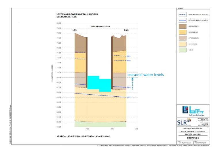
The above graphic shows to scale the LML depth, where the seasonal variation of water only fills 1/4 of the lagoon. This lack of water will go on in time to causes dryness and cracking in the walls of the lagoon, risks leakage into the upper aquifer and contaminating it.
